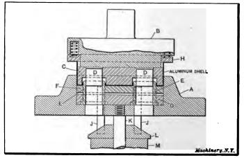
Fig. 18. Combination Piercing and Ribbing Dies
